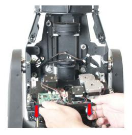
6. Loosen the thumb screws for the gobo wheel module, and carefully slide the gobo wheel module out of its mounting slots. Place the module on a flat, stable surface in a **DUST-FREE, INDOOR** location.
